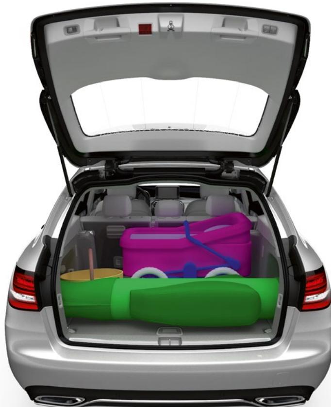
**FIGURE 3** Packing study with arbitrary objects: The TrunkPacker automatically finds the only possible placement of the green golf bag using the lateral cavities; for the brown shopping basket and the pink buggy the requirements are met to only assume upright orientations (© Daimler)
