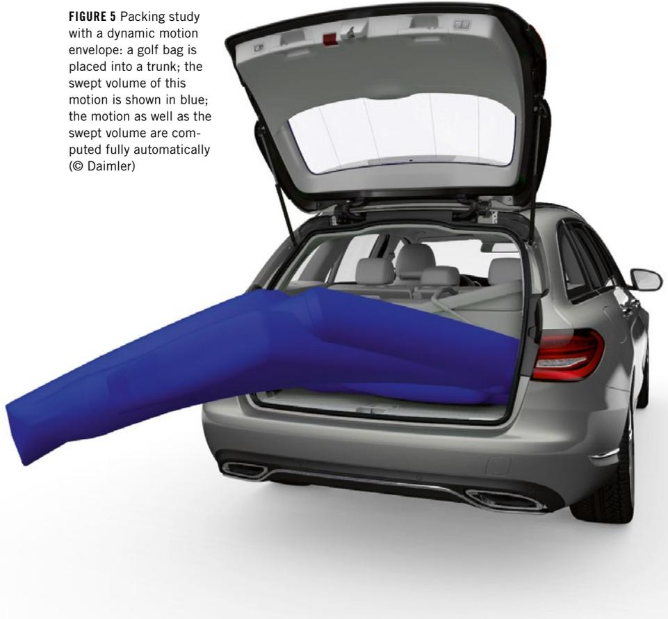
nents [3]. The developed methods in these areas will help to further optimise the computer aided design of trunk geometry.
