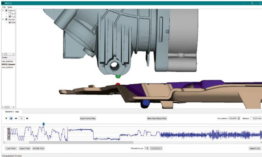
**FIGURE 3** Screenshot from the Melvis software: focussed calculation of the minimum distance between two components during a movement; the red and green dots indicate the spatial positions on the components that realize the distance for the current point in time (top); the blue graph shows the temporal evolution of the minimum distance during the movement (bottom) © Daimler
