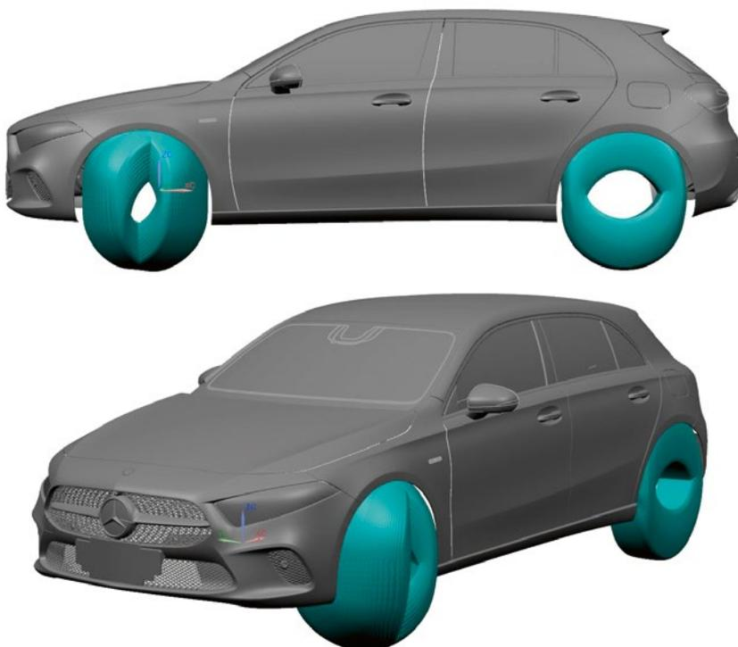
**FIGURE 4** Motion envelopes of front and rear tires: the space occupied by a tire is represented by a motion envelope © Daimler
