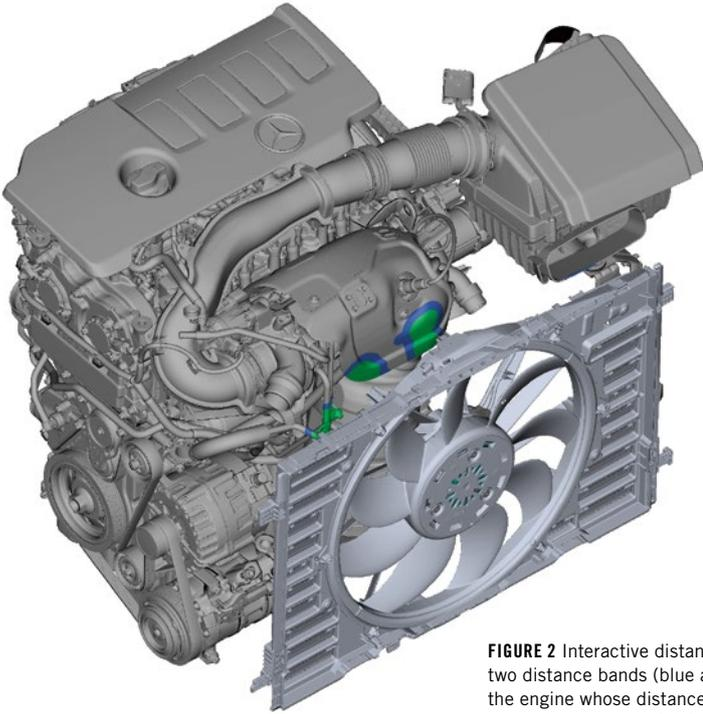
**FIGURE 2** Interactive distance band analysis with two distance bands (blue and green): areas of the engine whose distance to the fan lies within a certain range are highlighted; the width of the bands and the motor position can be changed interactively (© Daimler)
